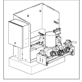
**6.** Pass 3/8-16 UNC button-head socket cap screws through the square panel hole in the side walls of the case and through the corresponding slot in the drive unit.
