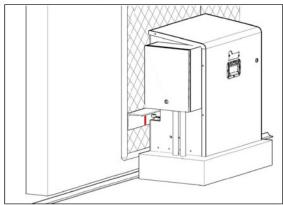
the gate towards the fully opened position at full speed. Press the stop button a few feet before fully opened position. Roughly measure the coasting distance from where the stop button was pressed and where the gate came to rest. Use this as your distance to mark the offset line.
