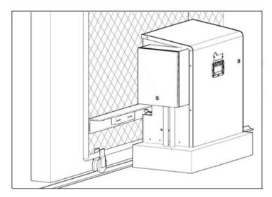
Installing the limit blocks and adjusting the limit switches is most easily done after the case has been mounted and before the drive is placed into the case / enclosure. Final adjusting the stop blocks should be done with the gate powered by the operator.
